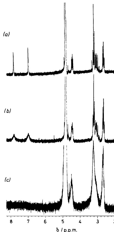
FIGURE 6 Proton n.m.r. spectra of 2 \times 10^{-2} mol \text{dm}^{-3} carnosine in \text{D}_2\text{O} at pH 7.2. The concentrations of added \text{Cu}^{2+} are (a) 0, (b) 2 \times 10^{-5} , and (c) 2 \times 10^{-4} mol \text{dm}^{-3} . The large resonance at ca. 5 p.p.m. arises from HOD. Full assignment of the spectrum was reported by Ihnat and Bersohn 18
